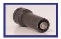
**Spring Magnet.** These types of sockets have the magnet mounted to spring. This allows the magnet to move with the fastener as it is being driven down. Most sockets can be ordered with the spring magnetic option. This option is designated by adding SM to the end of the part number.
