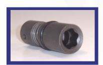
**Wobble Socket.** This unique design gives any surface drivesocket an additional fifteen degrees of travel. The additional travel allows the socket to position on the fastener quicker. Different then a traditional universal the design allows for disassembly in a matter of seconds allowing the working end to be replaced. Wobbles are available in 3/8, 1/2, 5/8 and 3/4 inch drive sizes.
