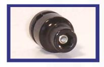
**Tube Magnet.** These types of sockets are used when the application requires the fastener to travel into the socket i.e., a stud bolt combination. The tube magnet holds the nut while allowing the stud to travel into the socket. Most sockets can be ordered with the tube magnet option. This option is designated by adding TM to the end of the part number.
