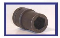
**Fast Lead.** These types of sockets are designed to work with multiple spindle power tools. The design allows the socket to engage the fastener while moving. Most sockets can be order with the fast lead option. This is designated by adding FL to the end of the part number.
