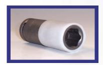
Rotating Sleeve. These types of sockets offer two advantages. Similar to the fixed sleeve socket it will reduce the potential of damage to a painted or chromed surface. Additionally, the sleeve rotates so there is less of a chance of injury to the operator. This unique design will not allow loose clothing, or gloves to be entangled into a spinning socket. Many Lance sockets can be ordered with a rotating sleeve option. This option is designated by adding RS to the end of a part number.
